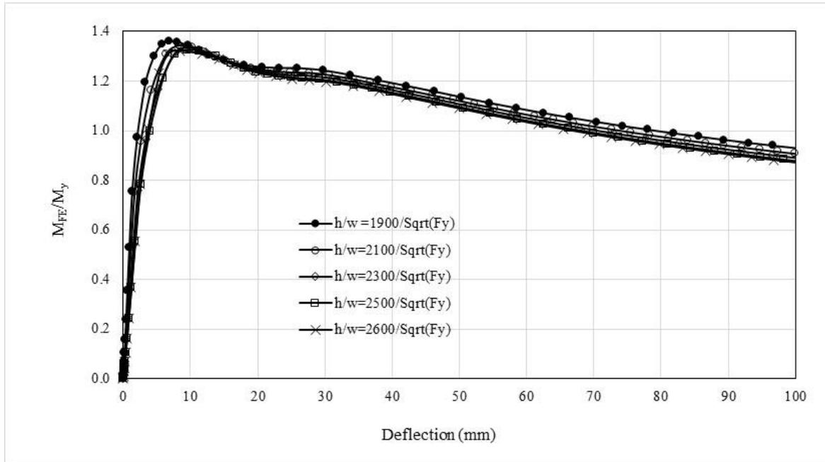
Figure 9: Effect of beam web slenderness on moment capacity with Class 3 flange
