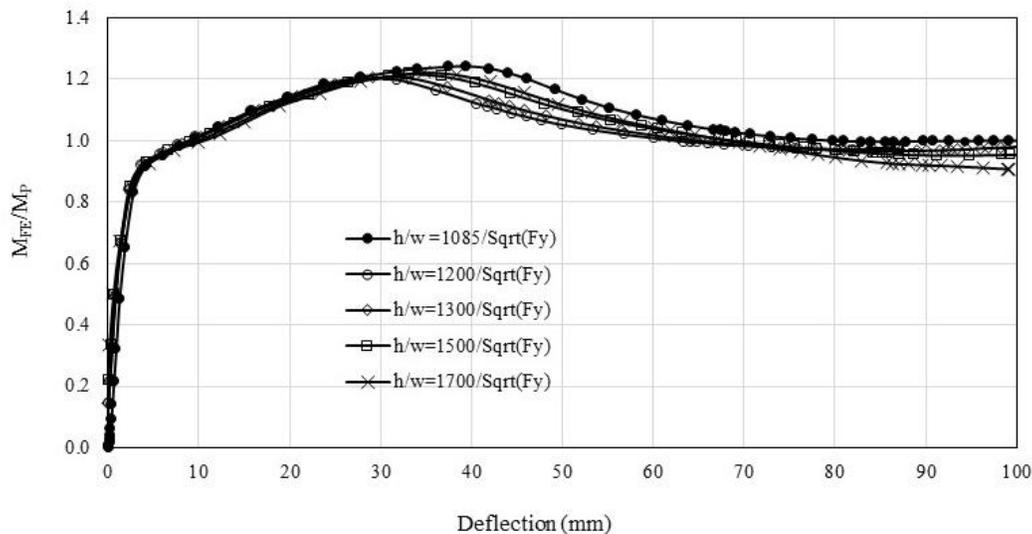
Figure 8: Effect of beam web slenderness on moment capacity with Class 1 flange
