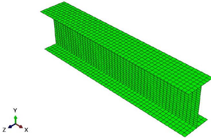
Figure 2: FE Mesh for configuration of finite element model
