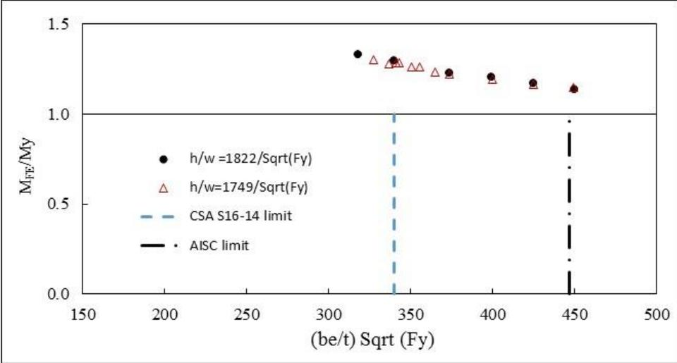
Figure 7: Effect of flange slenderness for beams with Class 3 web
