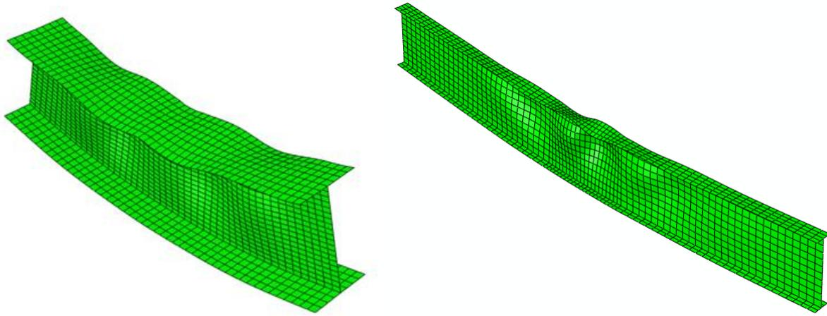
Figure 4: State of specimens at local buckling (FE model PK-4 left and FE model WS-3 right)
