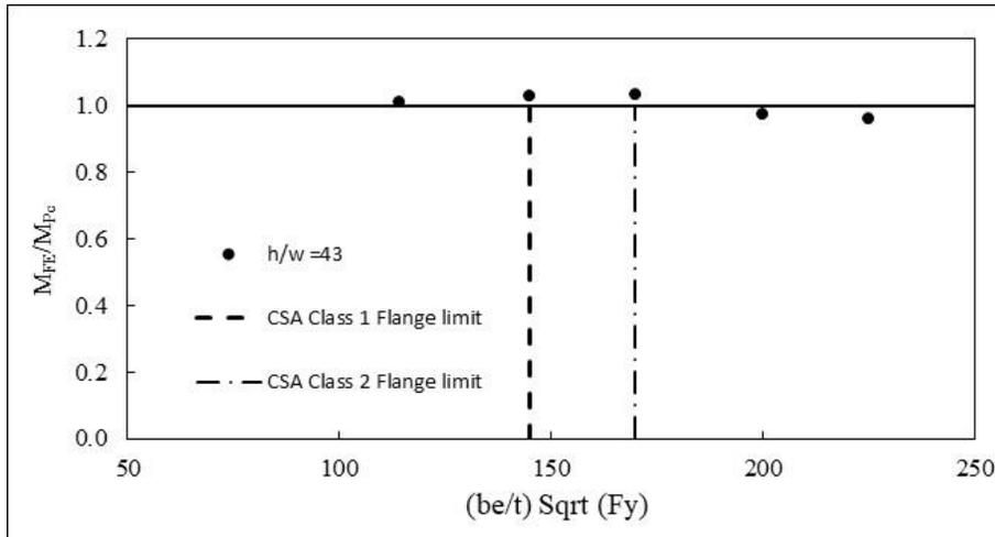
Figure 10: Effect of flange slenderness on moment capacity of beam-columns with Class 1 web
