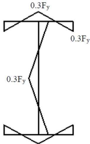
Figure 3: Typical residual stress pattern (Chernenko and Kennedy 1991)
