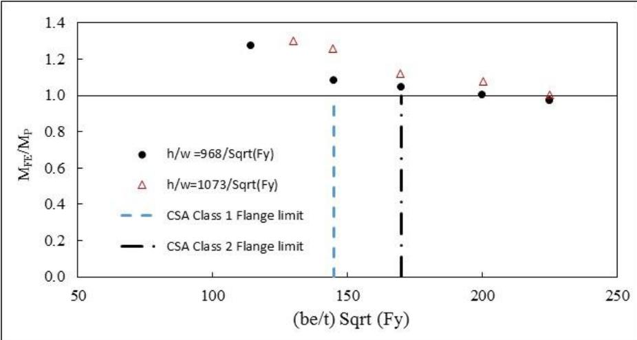
Figure 6: Effect of flange slenderness for beams with Class 1 web
