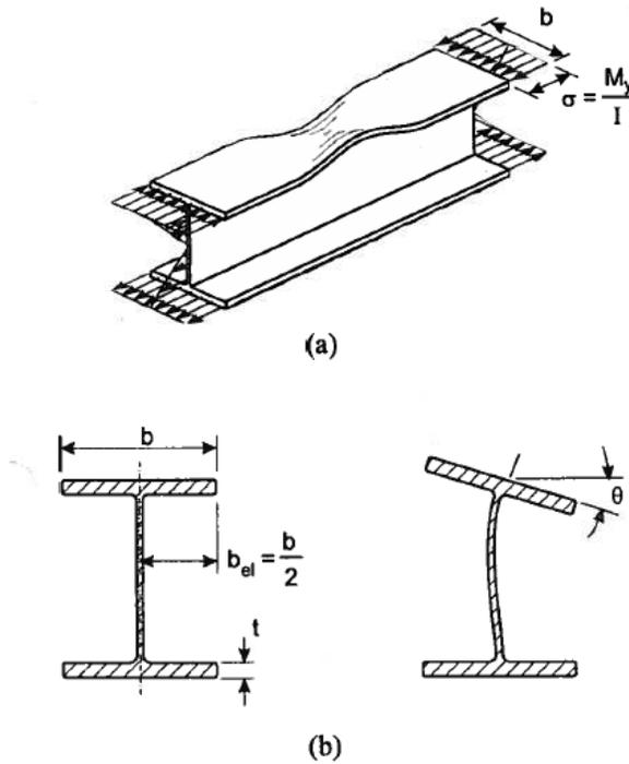
Figure 1: Typical local buckling mode of W-shape member (Kulak and Grondin 2018)
