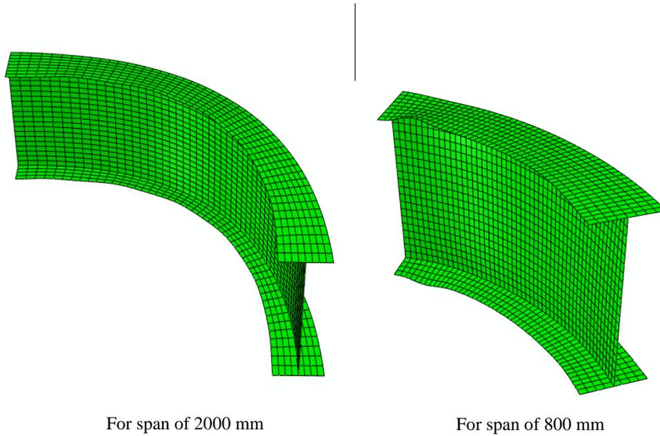
Figure 5: FE mesh of W530x74 section under weak-axis bending for different spans
