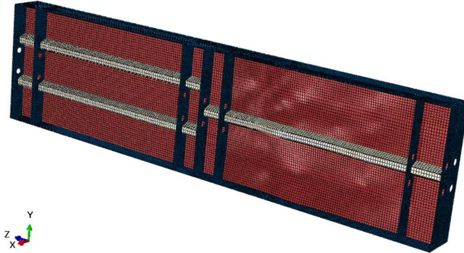
**Fig. 13:** Finite element model with geometric imperfection.
