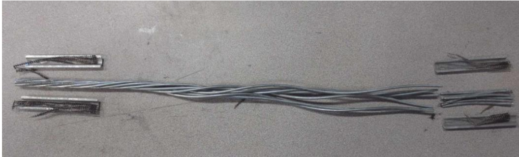
Figure 5: Fracture and unraveling of messenger wire during testing
