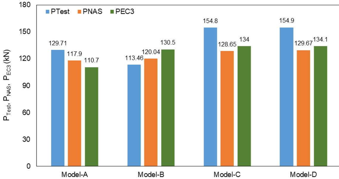
Figure 8: Comparison of test results with the design strength predictions
