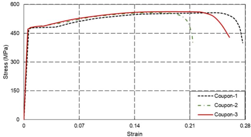
Figure 2: Stress vs. strain behavior of the coupons
