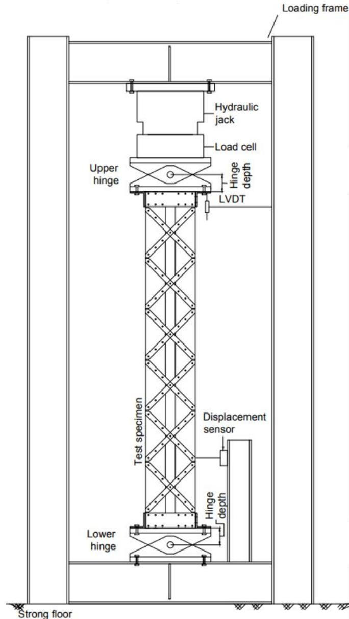
Figure 3: Details of the test set-up
