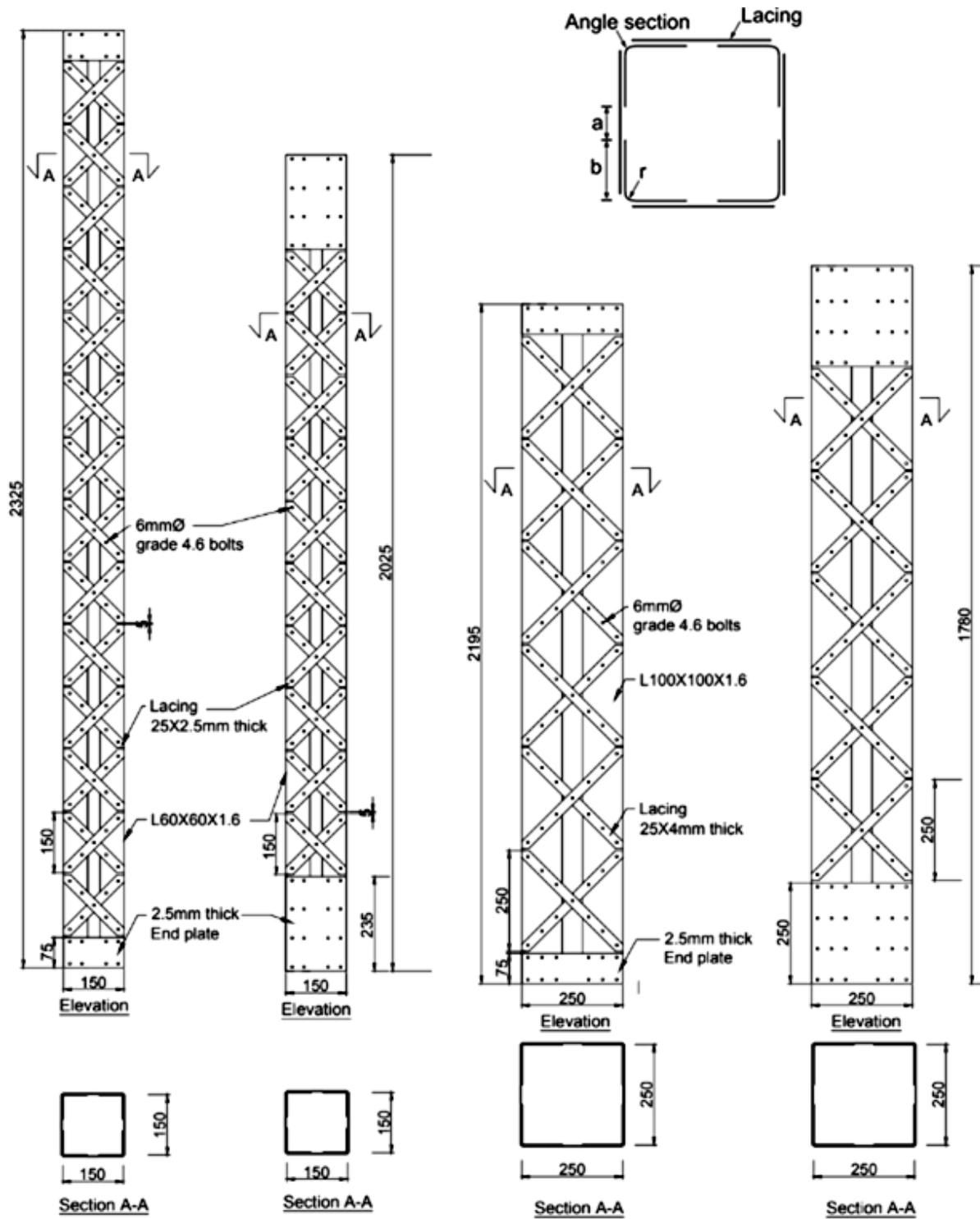
Figure 1: Details of the test specimens
