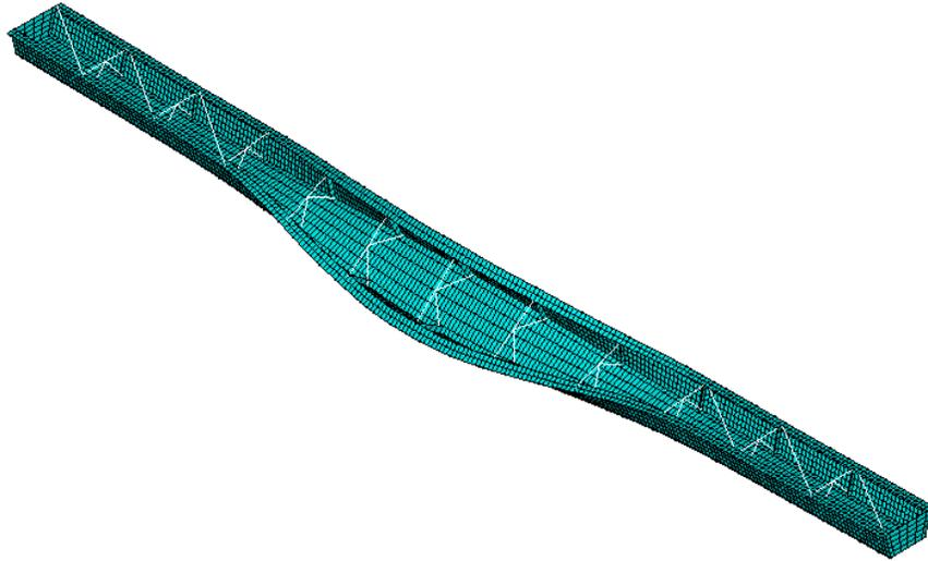
Figure 1. FE model of the buckled box girder
