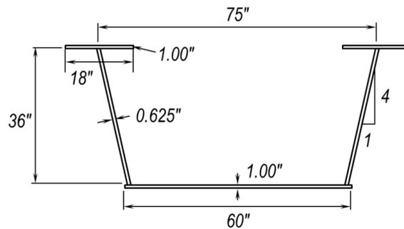
Figure 2. Geometric Parameters of the Box Girder Section
