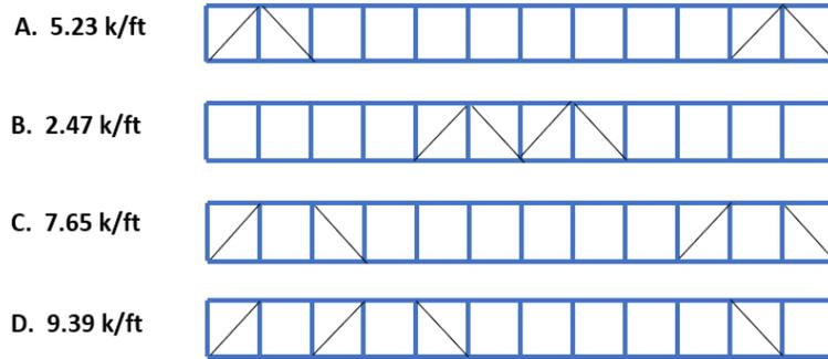
Figure 8. Comparison of the Buckling Load for 4-diagonal Configurations
