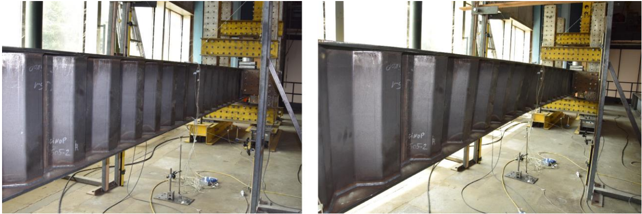
Figure 7: Lateral-torsional buckling failure (LTB) of specimen 1/1
