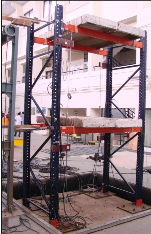
Figure 3: Steel pallet rack mounted on a shake table
