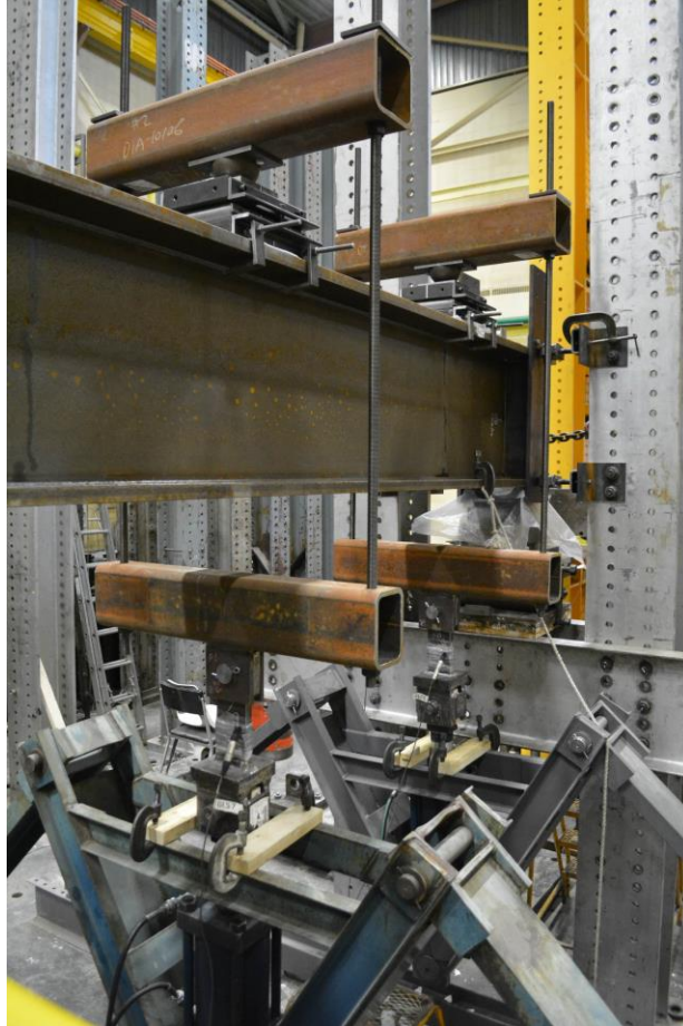
Figure 4: Gravity load mechanism
