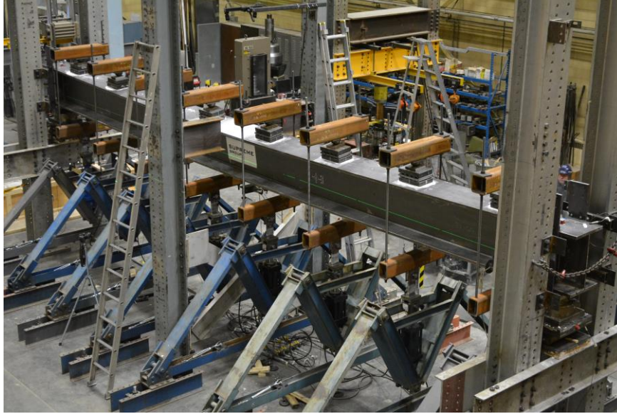
Figure 9: Buckled SP2-2 at the end of the test
