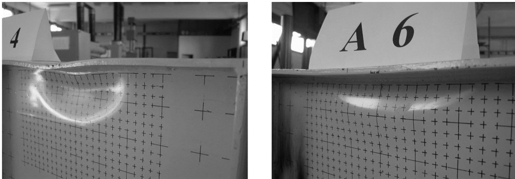
Figure 4: Failure mode for stiffened girders A4 ( s_s=25 mm) and A6 ( s_s=125 mm)
