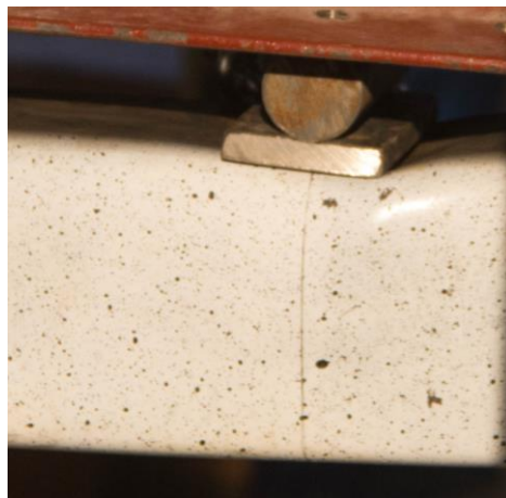
(a) Local failure of S900-10-3
