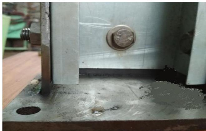
Figure 6: End condition to allow warping
