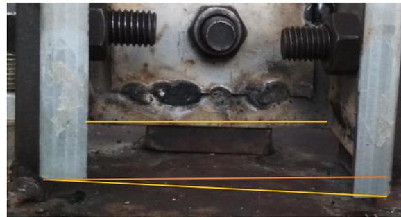
Warping deformation at bottom
