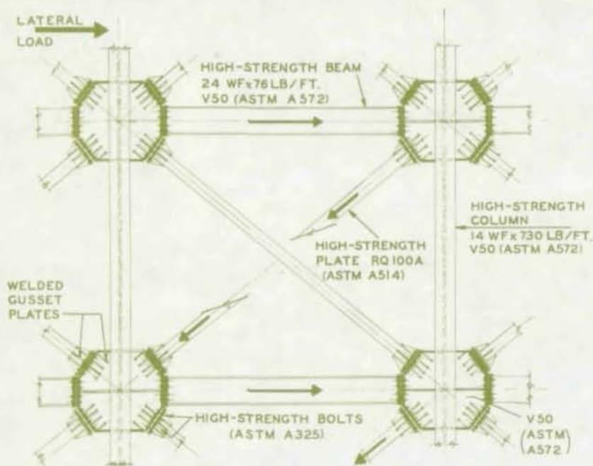
Arrows in detail indicate line of load transmission through framework when a high lateral load is applied.
