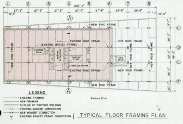
Although the working stresses in many of the existing columns were larger than those used in the design of the original building, relatively little column reinforcement was required. This is primarily because higher weak and strong axes bending stresses are permitted for steel columns in today's AISC Specification than were permitted in 1958. In addition, the steel columns were found to conform to ASTM A36 requirements, even though A7 material was originally specified.
