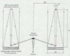
Schematic of optical layout - (section is through two of six telescopes).
