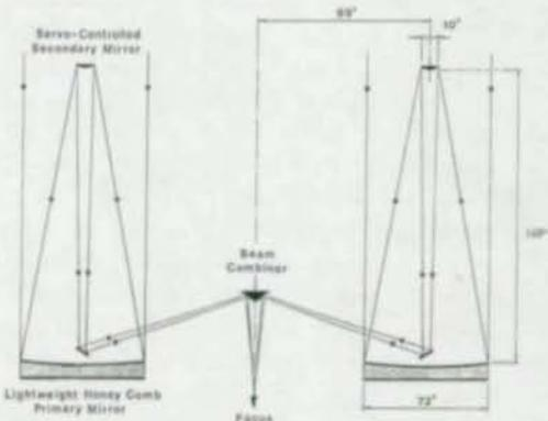
Schematic of optical layout - (section is through two of six telescopes).
