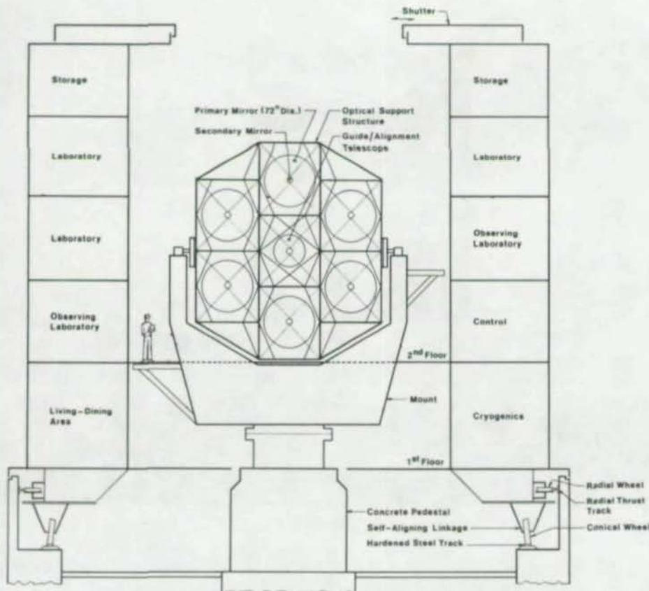
Schematic of Multiple Mirror Telescope and rotating building.
