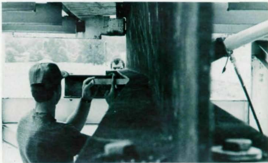
Steel ram swings against structure to simulate damage to overpass girders. Damage is assessed (r).
