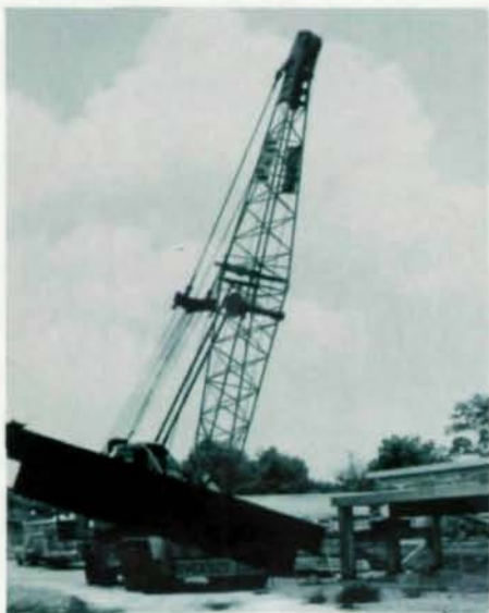
Steel ram swings against structure to simulate damage to overpass girders. Damage is assessed (r).
