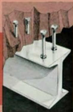
**Composite Bridges** – Shear connectors provide equal shear in all directions, eliminate distortion that might result from hand welding and permit more satisfactory compaction of concrete around the connectors.
