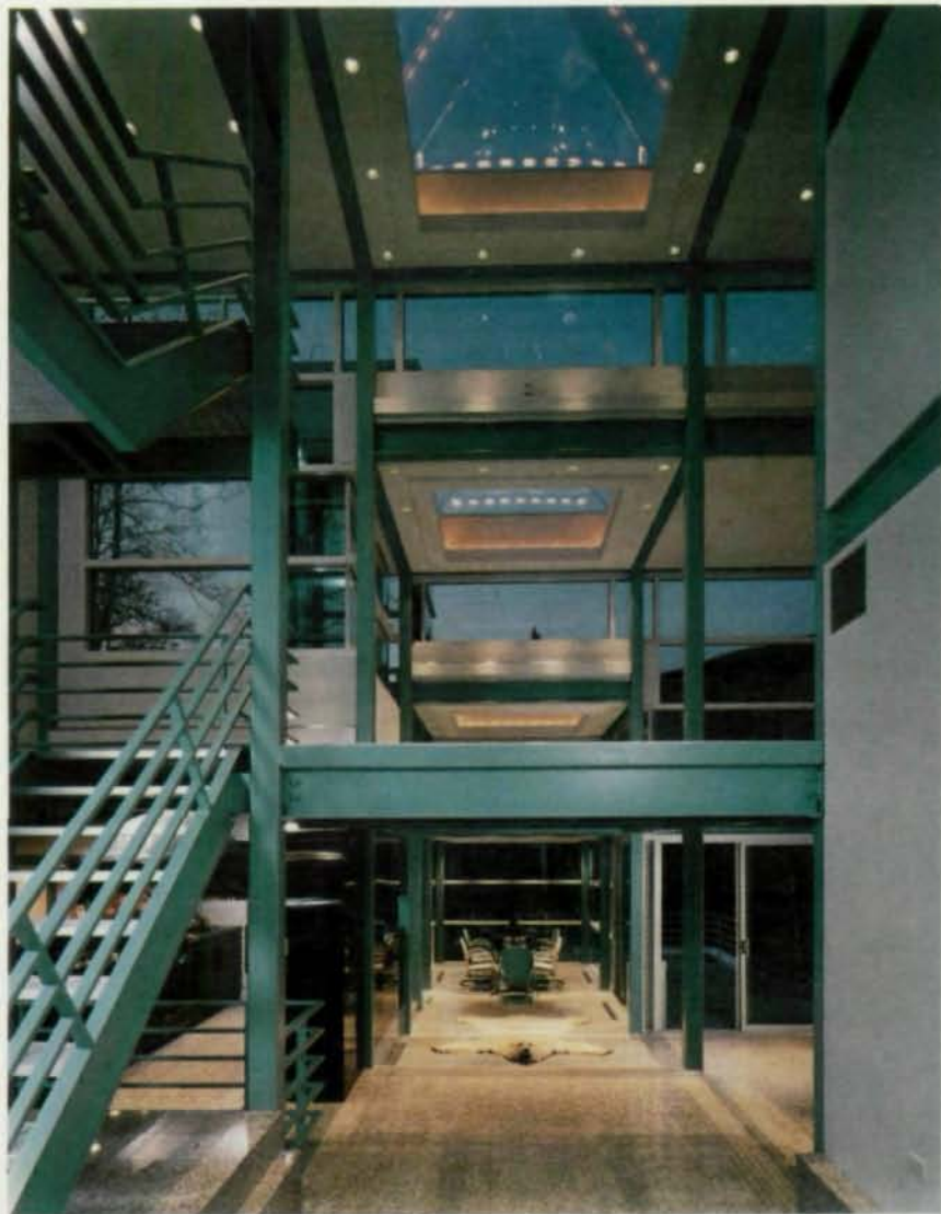
Steel was left exposed on the inside in order to give visitors an understanding about the methodology and construction of the home.
