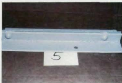
Angle from steel bridge railing after application of candidate upgrade system.
