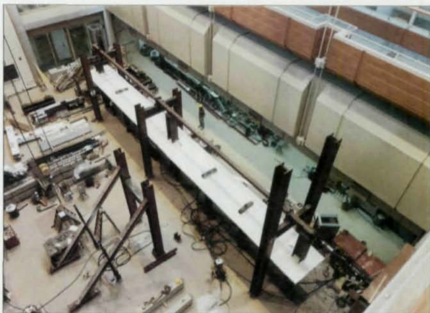
Pictured above is another view of the full-scale, two-bay, one-story subassembly allowing the testing of a type of semi-rigid connection.
