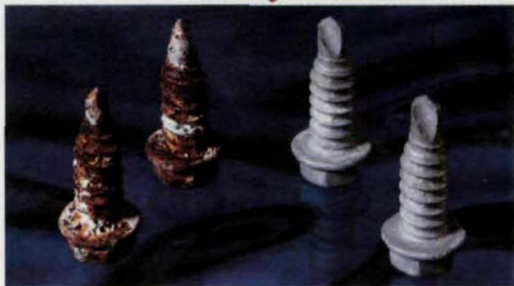
Fasteners, left, finished with standard mechanical zinc. Right, finished with mechanical zinc plus Magni coating system. Unretouched photo, after 5 cycles of Kesternich testing.
