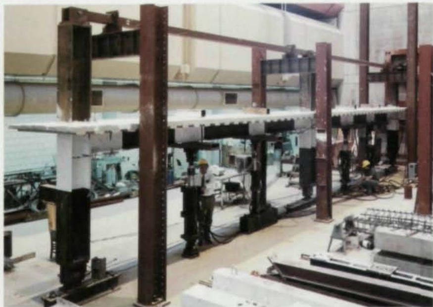
Pictured above is a full-scale, two-bay, one-story subassembly allowing the testing of a type of semi-rigid connection.
