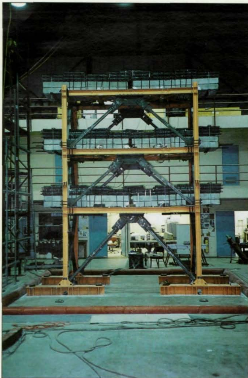
Pictured above is the assembled three-story, one-bay test structure supporting 30,000 lbs. per floor and standing more than 20-ft. high. The assembly featured moment resisting frames and Chevron braces connected with steel-on-brass SBCs at each level and on each of the two frames of the structure.
