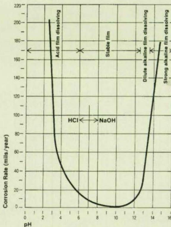
Effect of pH value on the corrosion of zinc
