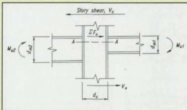
In checking panel zone web shear in a column member why is  $M_1$  defined as the sum of the lateral load and gravity load moments on the leeward side of the connection, and  $M_2$  defined as the difference between the lateral load and gravity load moments on the windward side of the connection? It seems to us that the difference of moments apply on the leeward side and that the sum of the moments should apply on the windward side.
