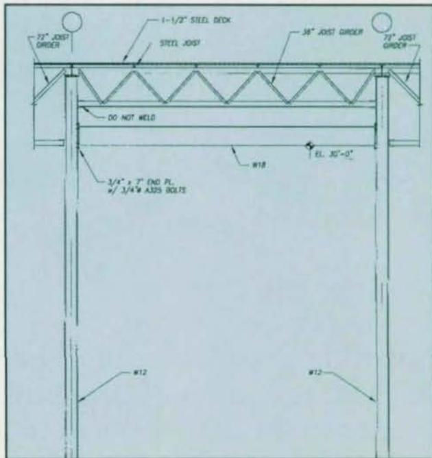
The roof member in the 24-ft. bay is a pin-ended joist girder. The rigid frame is created with an end-plated wide flange beam located to align with the bottom chord of the deeper joint girder in the adjacent 72-ft. bays. This arrangement shortened the effective height of the rigid frame column and simplified the connections of both the joist girder and the wide flange beams, without limiting the 30-ft. clear height in the building, a crucial requirement given the structure's function.
