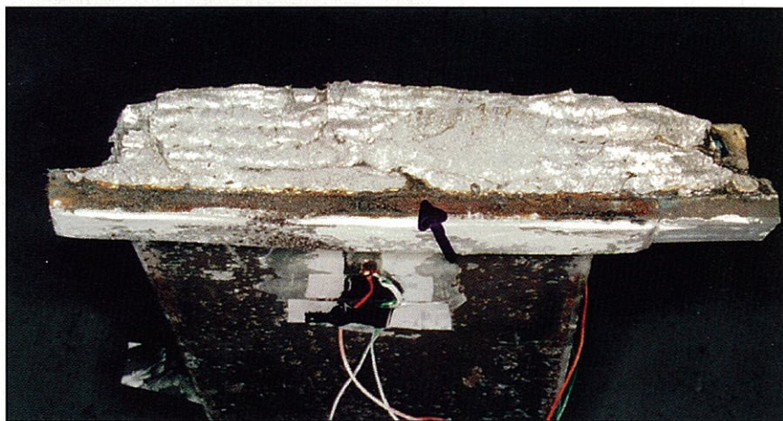
Figure 5a: (top) "Pre-Northridge" simulated beam flange to column test fracture
