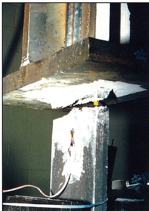
Figure 5a: (top) "Pre-Northridge" simulated beam flange to column test fracture
