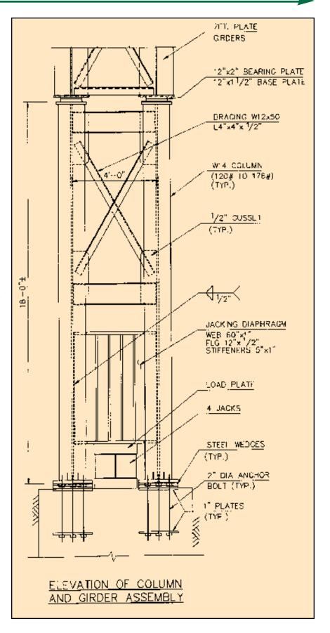
to 30-ft.-3-in. The web plates were a uniform 6-ft.-10-in. by  $^{11}/_{16}$ -in., minimizing the intermediate stiffeners required. Flanges were 20-in. wide, with thicknesses varying from  $1^{1}/_{8}$ -in. to  $2^{7}/_{8}$ -in. There was at most one transition in thickness. Simple end conditions were insured by providing curved bearing shoes. Due to the magnitude of the axial loads, any bending moment transmitted to the columns was undesirable.
