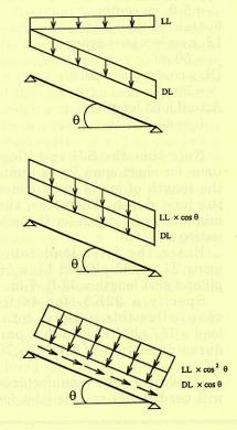
Joists are specified by their actual length and the load normal to the joist as the values that are used in the SJI load table. The dead and live loads for a roof system are typically oriented on two different axis.
