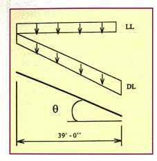
Example: Roof slope = 6:12LL = 14 psf DL = 22 psf Plan dimension of bay,
