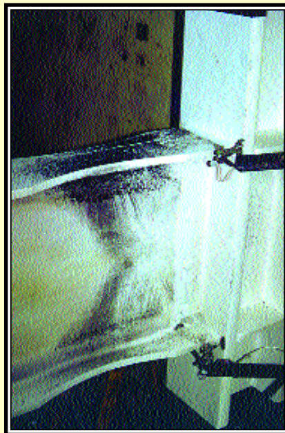
Figure 6a (above): View of beam flange of specimen DB4 at 0.012 rad. plastic rotation (column is at left)
