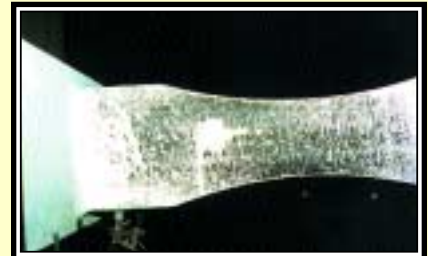
Figure 6a (above): View of beam flange of specimen DB4 at 0.012 rad. plastic rotation (column is at left)
