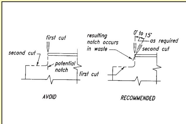
The *AISC Manual of Steel Construction Load and Resistance Factor Design, Volume II* (1994) recommends on page 8-225 that an approximate minimum radius to which the re-entrant corner of a beam cope must be shaped is  $\frac{1}{2}$  in. While there is nothing magical about a  $1\frac{1}{2}$ -in. radius, this value is recommended to emphasize that square-cut corners and significantly smaller radii do not provide the smooth transition required.
