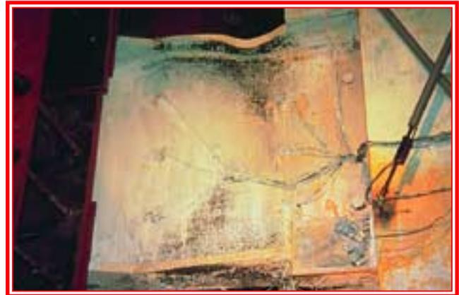
Shown is the weak axis connection with a W33x152 beam and W14x455 column.
