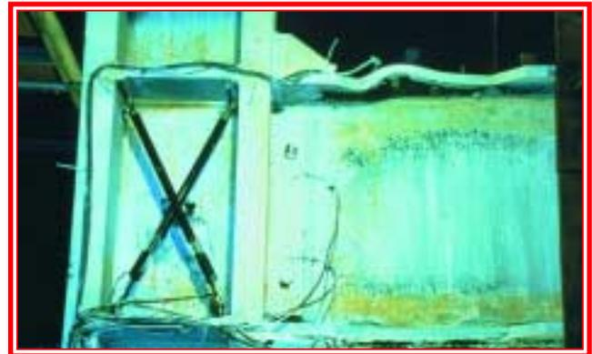
Shown is the strong axis connection with a W27x178 beam and W14x455 column.
