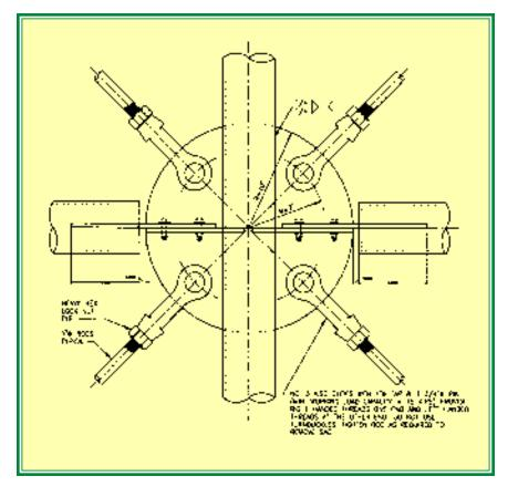
and two coats of architectural finish paint. To speed erection and maintain the integrity of the shop finishes, the design call for all field connections to be bolted. As a final precaution against corrosion, all bolts, clevises, pins and turnbuckles were hot-dip galvanized prior to field painting.
