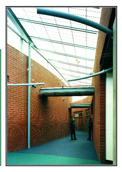
patrol functions, administrative space and a community room. While the building itself is masonry and concrete block, the roof structure is steel, as are the window lintels and some exposed architectural steel elementsmost notably an impressive walkway overhang.
