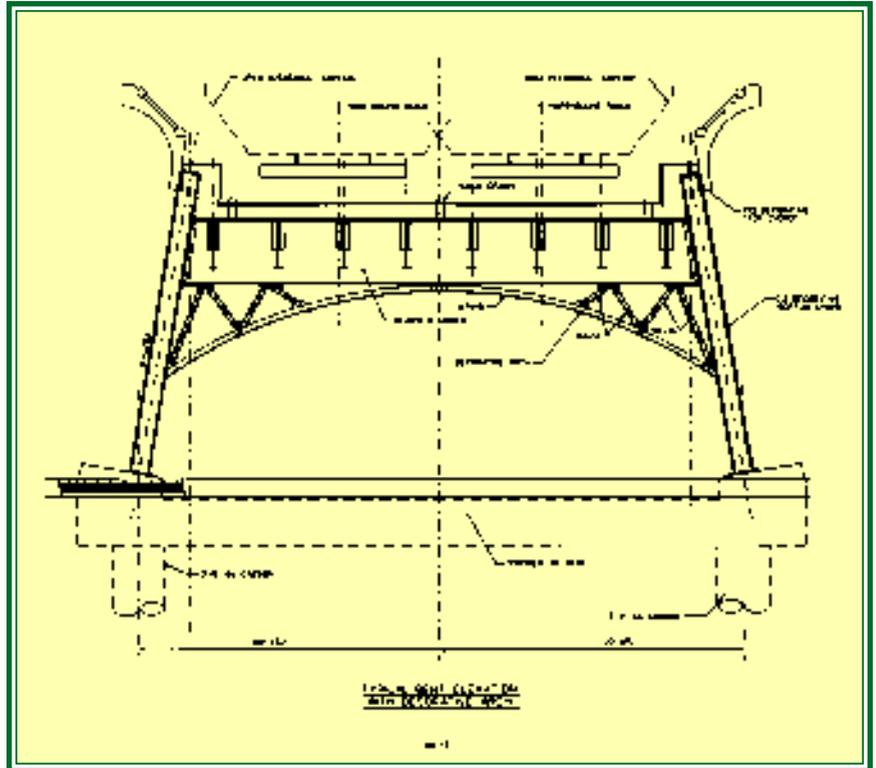
7th Avenue, 6th Avenue and the Mall between them. Limestone arches with 32’-tall lighted sentinel towers at the corners span the streets. A 19-span steel trestle connects the two “stone” arches. Shallow, graceful arches sweep the length of the bridge. Transverse arches springing across battered columns echo the form of the longitudinal arch. The architect used short spans, battered columns, and diagonal elements to recall turn-of-the-century trestles and trusses.
