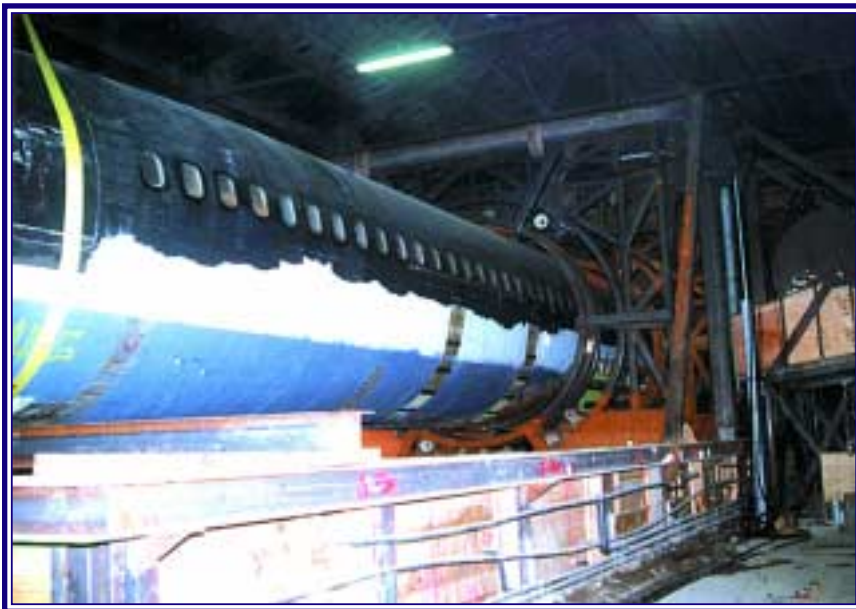
Pictured at top is the rotating gimbal during the water tank test. Shown above is the gimbal with the airplane fuselage installed.
