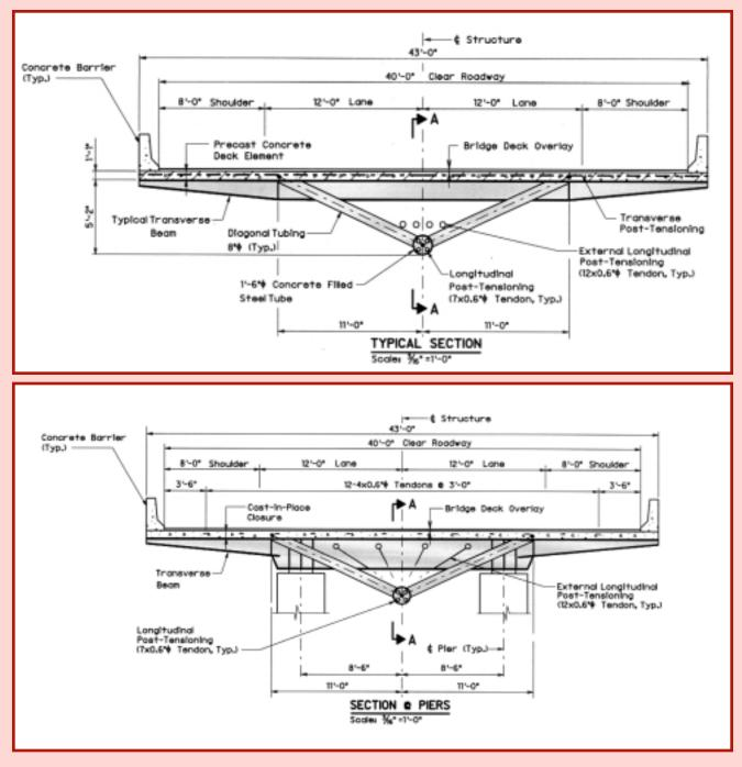
**Two-span Modular Space Truss**
