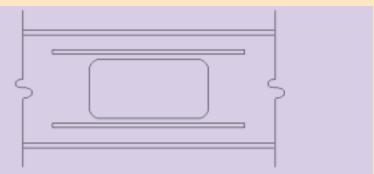
Figure 2. Web penetration reinforcement of an I-shaped beam.
