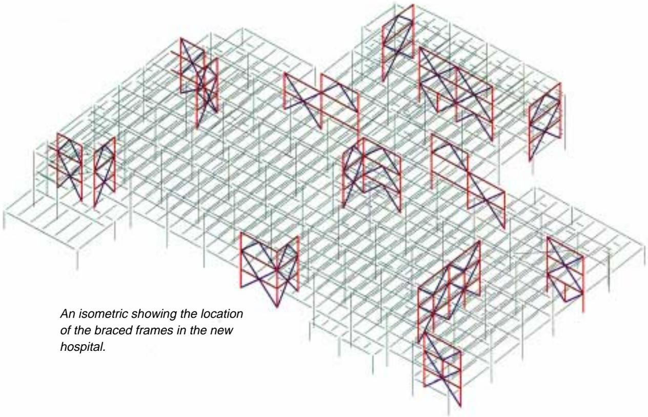
An isometric showing the location of the braced frames in the new hospital.
