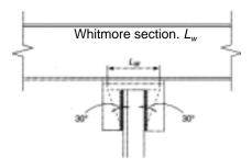
figure (below, left) for a WT hanger connection, the effective length for the Whitmore section  $L_w$  is determined using a spreadout angle of 30° along both sides of the connection, beginning at the start of the connection. It is applicable to both welded and bolted connections.
