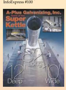
The "Supercoat," a lead-free hot-dip galvanizing kettle, offers pure high-grade zinc (99.9 pct pure) with a pure nickel powdermelt blend that helps prevent "gray-coat." The "Supercoat" gives an improved quality smooth/bright finish for an overall superior surface appearance, meeting the ASTM A-123 specification standard.
