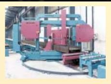
capacity and +40° to -30° miter capability. Features of the saw include robust twin column design, integrated NC miter setting and frequency controlled main drive. The KBS 1301 DG can be supplied as a stand-alone unit or in tandem with Kaltenbach's CNC Drilling Machines.
