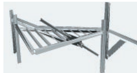
3-D rendering from Xsteel showing a portion of floor framing and structural bracing.
