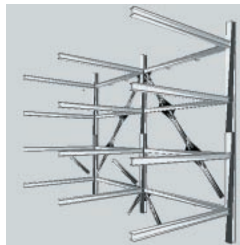
3-D rendering from Xsteel showing bracing.
