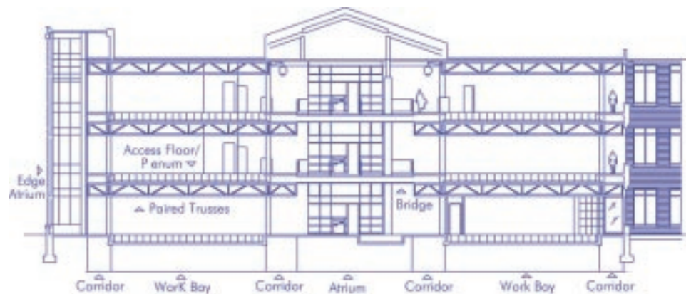
Building section showing central atrium flanked by work bays.
