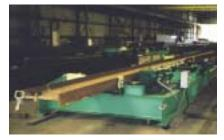
The CAMBCO high-capacity cambering machines cold camber wide-flanges and other steel beams. These four new models, 520, 825, 1170 and 1700, provide 25% more cambering power than CAMBCO's standard models. They can be used for cambering smaller beams for buildings or girders for highway bridges, in addition to straightening beams and tees.
