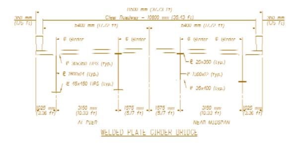
The steel alternate ultimately chosen for the Springview bridge features four lines of hybrid plate girders composed of 70 ksi HPS along with more traditional 50 ksi material.
