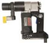
Wrenches are constant-speed, electric tools that have torque-multiplier attachments. With the torque-multiplier attachment each tool is able to fully pretension a wide range of bolts. For example: The Model STC 5AE, which weighs only 11 ½ lbs., will tighten 5/8" and 3/4" diameter structural bolts. Attach the multiplier and it will pretension both A325 and A490 bolts, up through 1-1/8" diameter.
