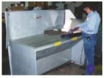
Dualdraw features air quality equipmentdowndraft tables for removing smoke and fumes away from operators' breathing zones.
