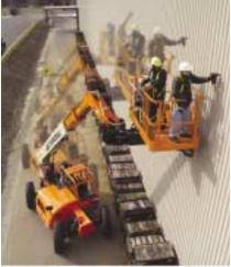
As a boom lift, a single operator can command all the functions of the machine, boom and platform. The platform has 500-lbs. unrestricted platform capacity at 43-ft. platform height and can be used on slope up to 10°. Used as a rough-terrain, telescopic-material handler the Transformer machine has a 42-foot maximum lift height with a 6,600-pound load.
