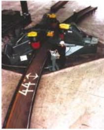
capacities from 10 ga. to 4" thickness and lengths from 2' to 30'; 4-roll double-pinch type plate bending rolls with capacities from 16 ga. to 4" thickness and lengths from 2' to 30'; beam benders with capacities of 44" beam and channel the "hard way" and the "easy way", 14" pipe, 16" round bar, 15" square bar, 24" x 12" flat bar the "easy way" and 24" x 6" flat bar the "hard way". Roundo also offers high speed, automatic plate bending rolls, flanging & punching machines and welding positioners.
