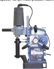
aluminum-die-cast mainframe, reversible-feed shaft for right- or left-hand operation, rearmounted control panel with LED load indicator, "One-Touch" cutter installation/removal—"no tools required", built-in motion detector—interrupts motor operation in the event of sudden machine movement, through-spindle coolant system enhances drilling performance while extending cutter life, accepts most popular brands of annular cutters, and accepts 3" DOC cutters for extended reach.
