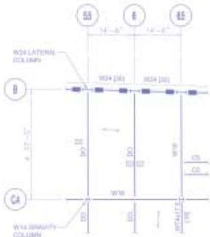
Typical 14'-6" floor framing module. This span allowed for an entire hotel unit to be constructed with its ceiling at the underside of the floor decking instead of at the underside of the W16 beams. This results in a 16" savings in headroom.
