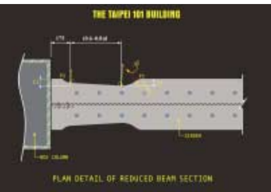
Above and below: At locations where plastic rotation would exceed 0.005 radian in a 950-year return period earthquake, reduced beam sections ("dogbone" cuts) increase moment connection rotational capabilities.
