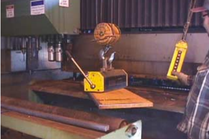
Large magnets and cranes can be used to manipulate large pieces of steel plate during fabrication.
