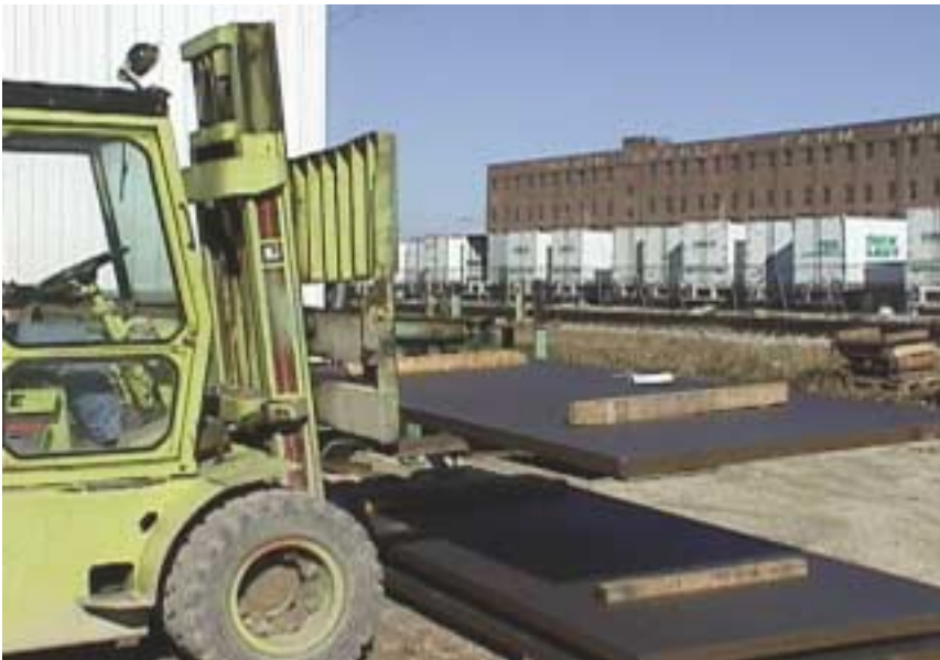
Fork trucks are commonly used to unload steel plate from flatbed trucks or rail cars. Plates must be carefully balanced to avoid handling disasters.
