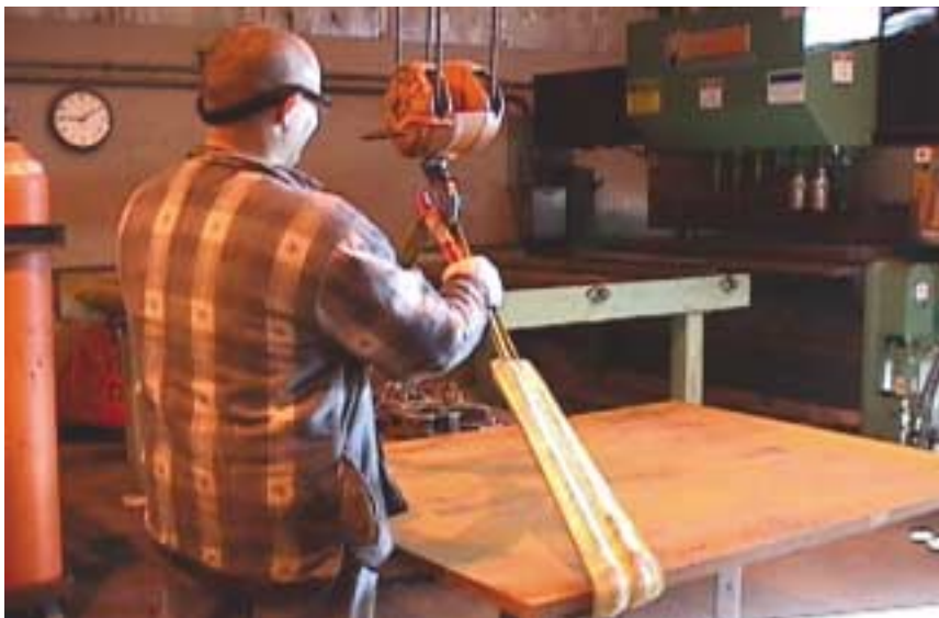
Special alloys require special handling to avoid marring the plate. In this case, a heavy-duty, cord-like strap is used during handling.
