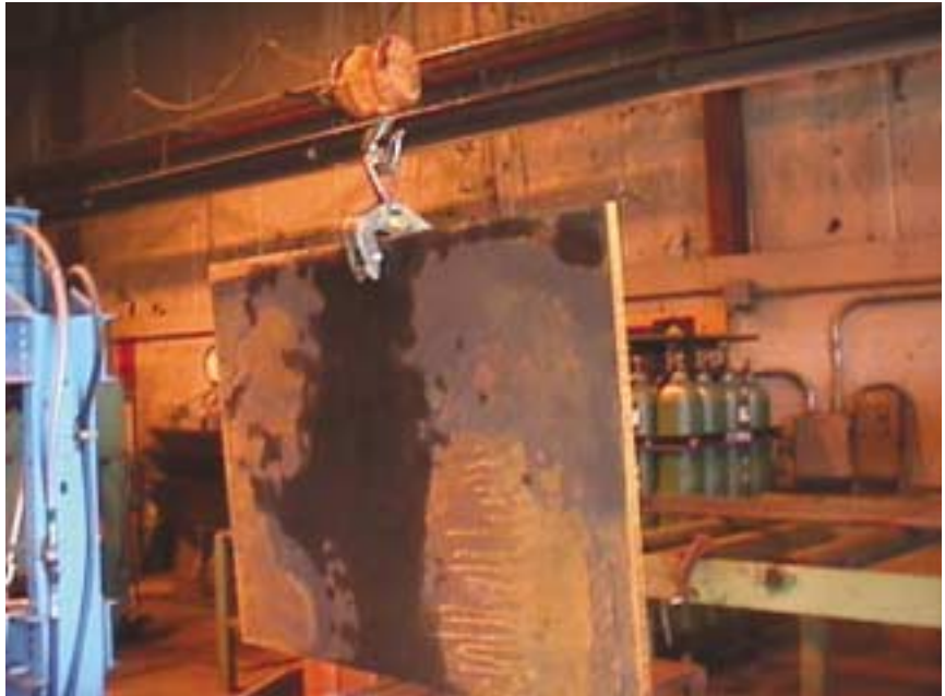
C-type clamp "dogs" are commonly used to grip the width of the plate for hoisting. The weight of plate material quickly adds up: a 10' by 10' by 1"-thick steel plate weighs over two tons.
