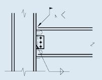
For joints in special moment frames, inelastic deformations in beams and column panel zones are more reliably attained with ASTM A992 wide-flange shapes. n just five years, ASTM A992 50 ksi steel has become the dominant material specification for wide-flange shapes, solidly displacing ASTM A36 wide flanges. In fact, ASTM A992 is so commonly rolled that it now costs less than ASTM A36 wide-flange shapes—and you would be hardpressed to find an ASTM A36 wide flange with a yield as low as 36 ksi.
