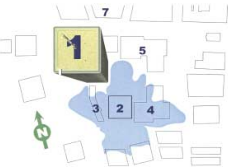
Figure 5. Pattern of heavy debris after the collapse of Tower 2, as mapped by LZA Technology.
