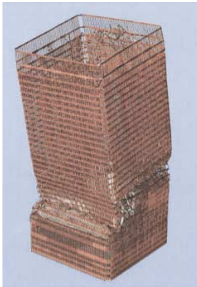
Figure 2. One frame from the computer model of the initiation of the collapse of Tower 2 performed by Weidlinger Associates.
