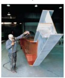
"And the paint reacts quickly, so you can apply a thicker membrane in a single application if you want, and put the whole coating down in one shot."
