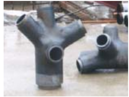
Forked supports for the VW-Skoda plant in the Czech Republic.
