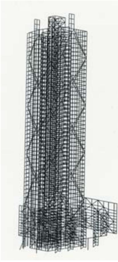
A three-dimensional computer model of the lateral system was generated using SAP2000 structural analysis software.
