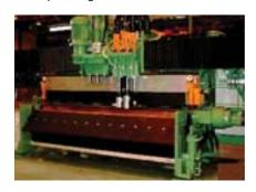
The FDB 2500/3 can process stock mill plate up to 96" wide, up to 3" thick, and up to 20' stock lengths. In a one-pass process, this machine can prepare all holes, carbide-mark the part number, and thermal-cut any shape or contour required.
